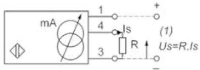
Ensure a minimum of 5 V between the + (terminal 1) and the sensor output (terminal 4)
