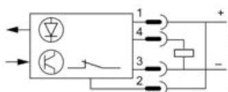
With output signal time delay (20 ms)
