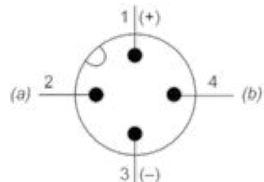
(a) Time delay: "OFF delay" of output signal: - no time delay: connect contact 2 to (+), - 20 ms time delay: connect contact 2 to (-)
