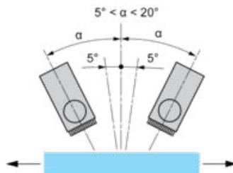
An angle of 5 to 10° from vertical is recommended for reflective or transparent surfaces Maximum vertical inclination: 20°
