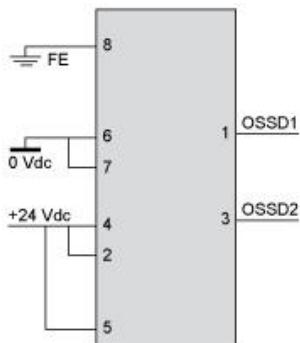
With External Device Monitoring (EDM) feedback loop
