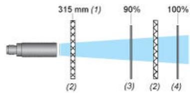
(1) : In reflex mode, the position of the reflector must be at least 315 mm away from the sensor.
