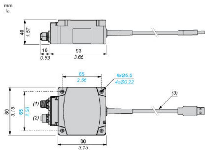
(1) : Male M12 connector, 5-pin: power supply
