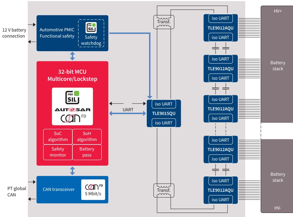
The battery management system is in charge of monitoring each of the cells included in a battery pack and ensuring that they are operated within the safe operating range.
