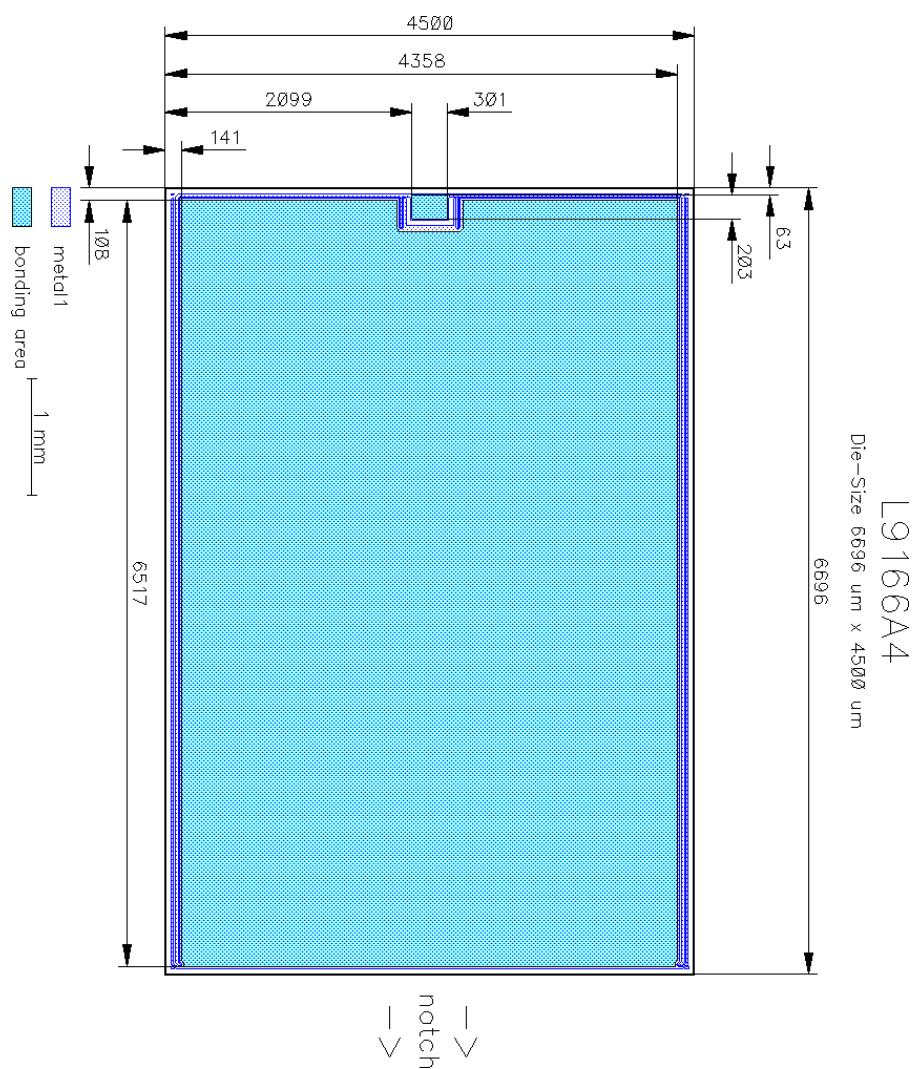
**Figure 1** Outline Chip, dimensions in  $\mu\text{m}$
